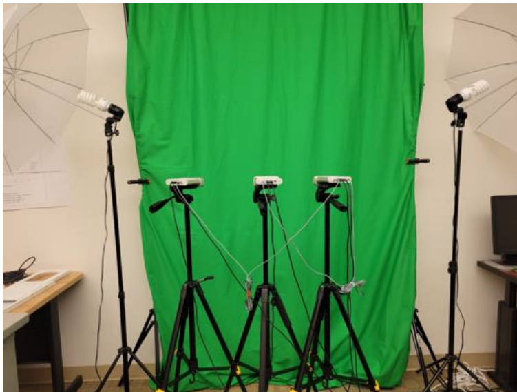
Fig. 2. This image represents the three Microsoft Kinect cameras with a green screen setup for real data collection.
